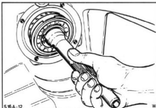
Fig. 138. Slide input shaft into housing.
