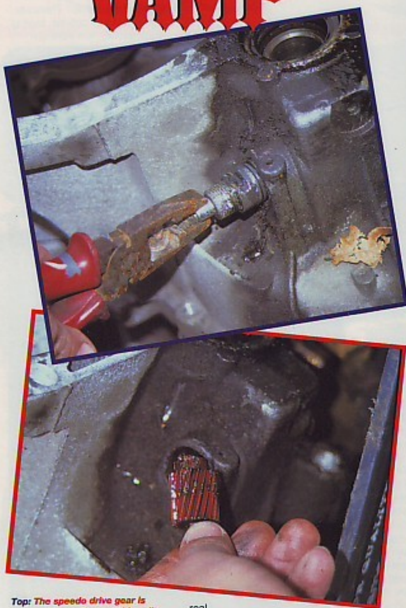
Above... then gently drawing the outer threaded bush out.
